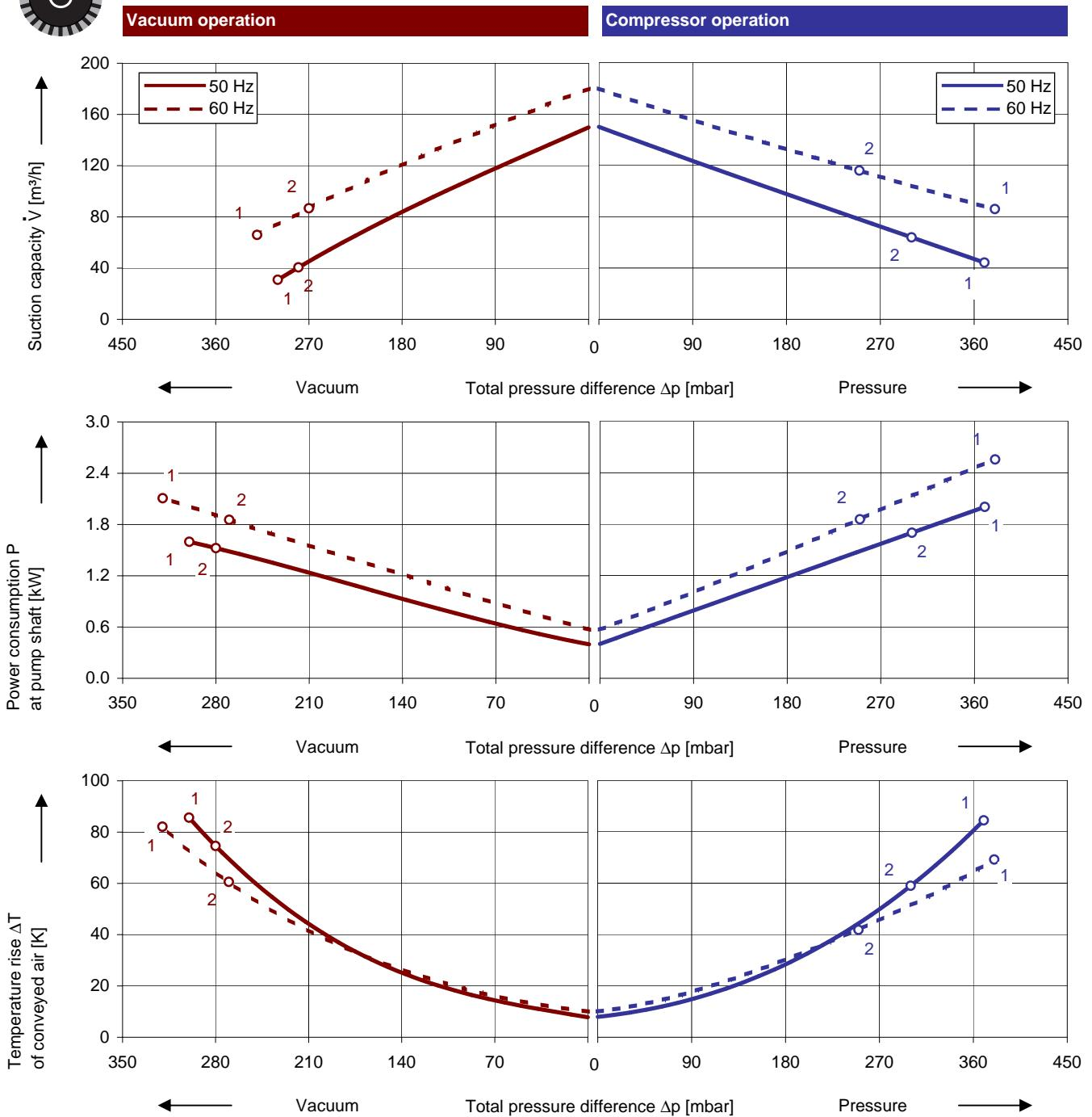
The performance curves are based on air at a temperature of 15 °C and an atmospheric pressure of 1013 mbar with a tolerance of  $\pm 10\%$ . The total pressure differences are valid for suction and ambient temperature up to 25 °C. For other conditions please get in touch with us.
