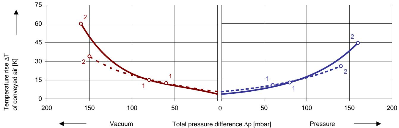
The performance curves are based on air at a temperature of 15 °C and an atmospheric pressure of 1013 mbar with a tolerance of  $\pm 10\%$ . The total pressure differences are valid for suction and ambient temperature up to 25 °C. For other conditions please get in touch with us.
