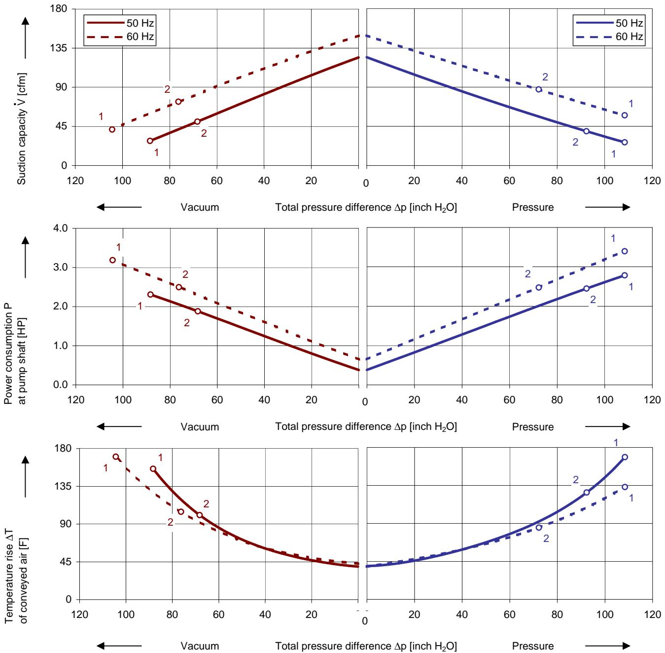
The performance curves are based on air at a temperature of 59 F and an atmospheric pressure of 401.53 inch H<sub>2</sub>O with a tolerance of  $\pm 10\%$ . The total pressure differences are valid for suction and ambient temperature up to 77 F. For other conditions please get in touch with us.
