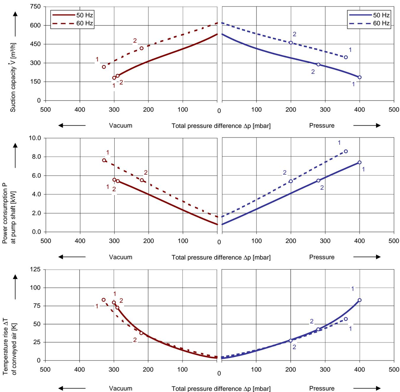
The performance curves are based on air at a temperature of 15 °C and an atmospheric pressure of 1013 mbar with a tolerance of ± 10 %. The total pressure differences are valid for suction and ambient temperature up to 25 °C. For other conditions please get in touch with us.
