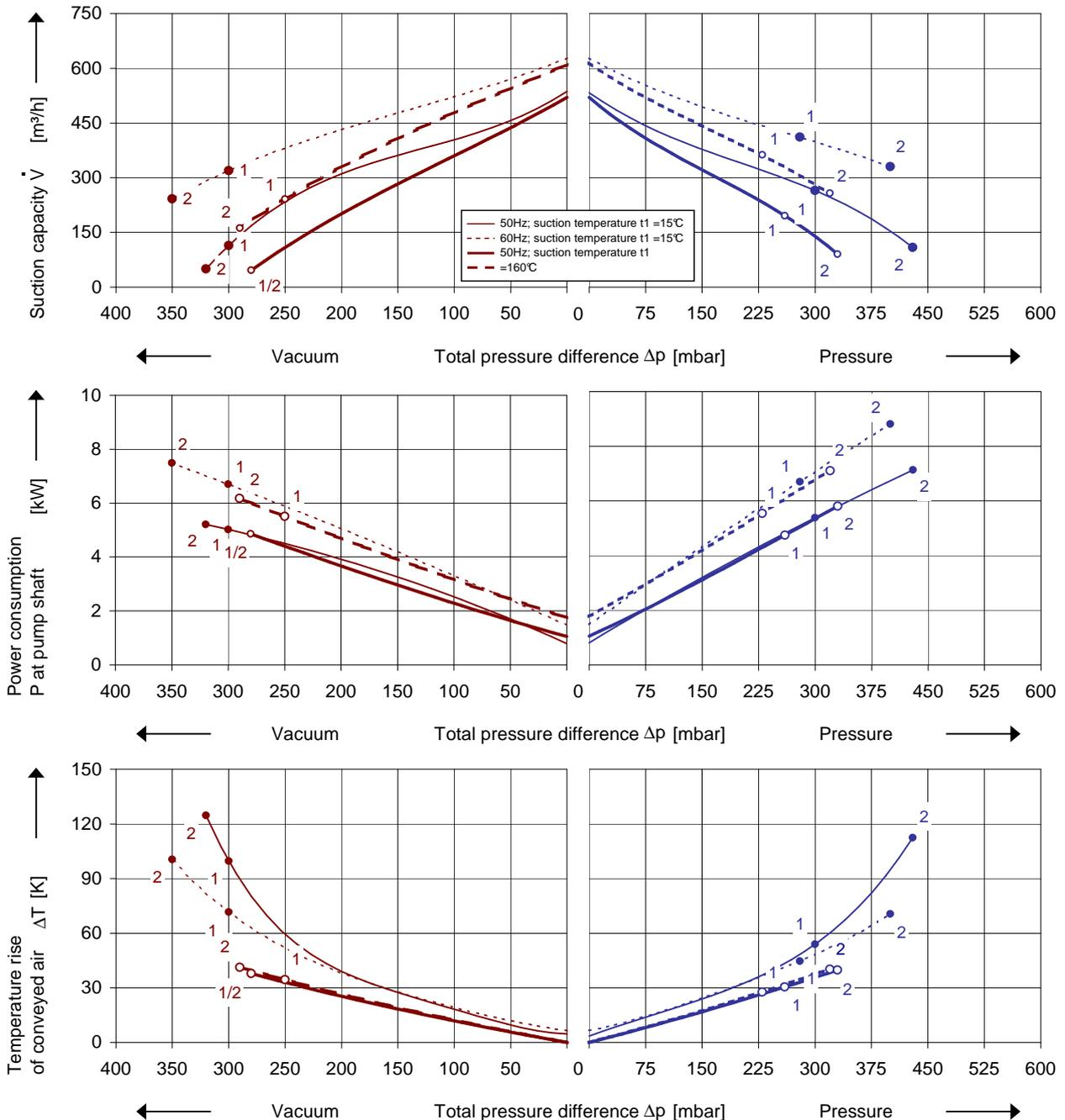
The performance curves are based on air at a temperature of 15 °C / 160 °C and an atmospheric pressure of 1013 mbar with a tolerance of ± 10 %. The total pressure differences are valid for suction and ambient temperature up to 40 °C. For other conditions please get in touch with us.
