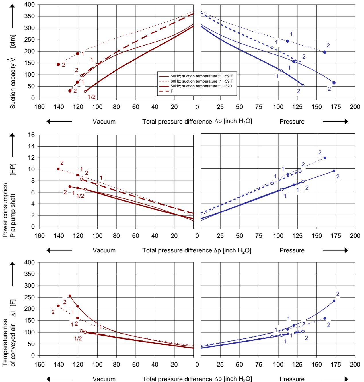
The performance curves are based on air at a temperature of 59 F / 320 F and an atmospheric pressure of 407 inch H<sub>2</sub>O with a tolerance of  $\pm 10$  %. The total pressure differences are valid for suction and ambient temperature up to 104 F. For other conditions please get in touch with us.
