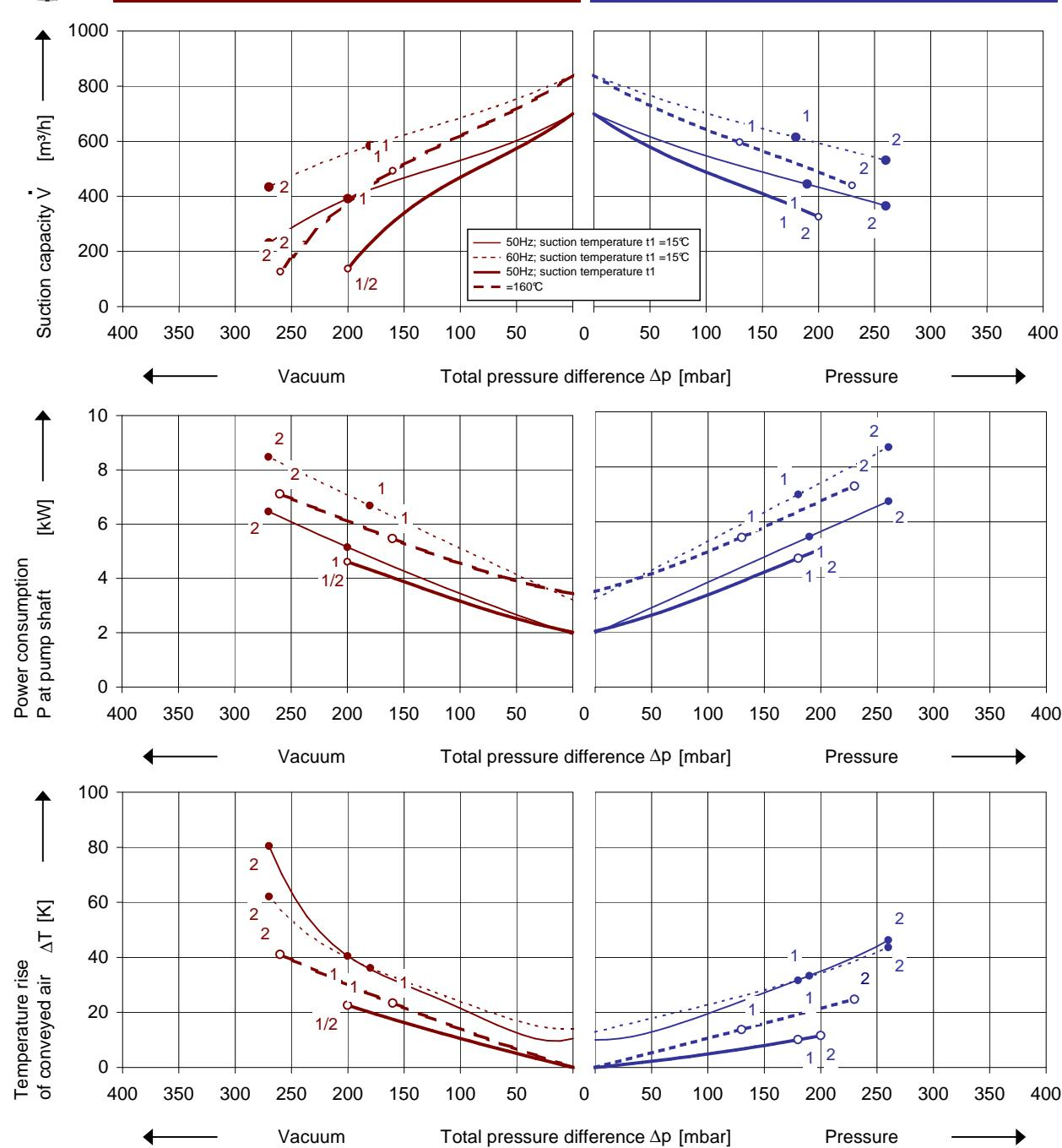
The performance curves are based on air at a temperature of 15 °C / 160 °C and an atmospheric pressure of 1013 mbar with a tolerance of  $\pm 10\%$ . The total pressure differences are valid for suction and ambient temperature up to 40 °C. For other conditions please get in touch with us.
