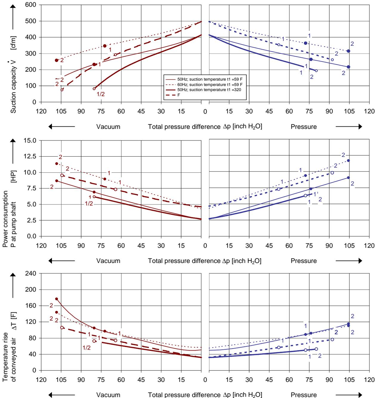
The performance curves are based on air at a temperature of 59 F / 320 F and an atmospheric pressure of 407 inch H<sub>2</sub>O with a tolerance of ± 10 %. The total pressure differences are valid for suction and ambient temperature up to 104 F. For other conditions please get in touch with us.
