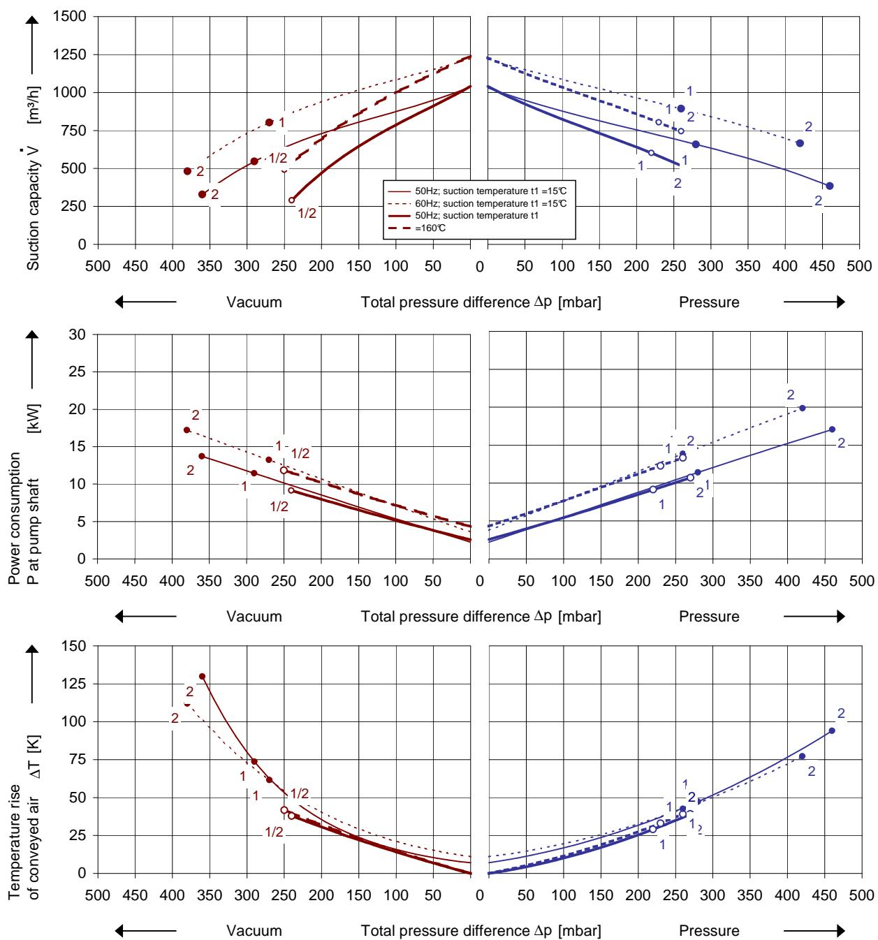
The performance curves are based on air at a temperature of 15 °C / 160 °C and an atmospheric pressure of 1013 mbar with a tolerance of  $\pm 10\%$ . The total pressure differences are valid for suction and ambient temperature up to 40 °C. For other conditions please get in touch with us.
