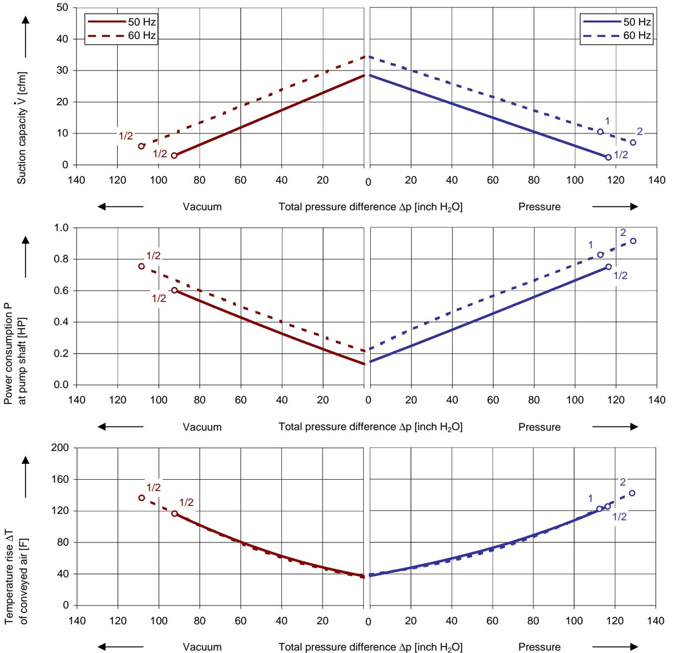
The performance curves are based on air at a temperature of 59 F and an atmospheric pressure of 401.53 inch H<sub>2</sub>O with a tolerance of  $\pm 10\%$ . The total pressure differences are valid for suction and ambient temperature up to 77 F. For other conditions please get in touch with us.
