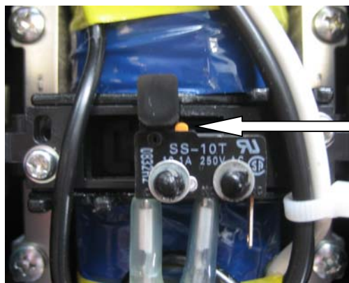
Photo 7/ 8: Diaphragm protection switch is activated
